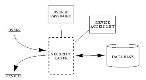
The explanation of the above example is that in an organization the information is gathered by the user like firstly the user sign 'sin in to his account by providing his ID and pass code then the process of the verification will be running internally and then authenticated by using the process of digital signature then the permission is granted to the user to access and gathering the information in the data storage. This is the security mechanism applied in the organizations.
